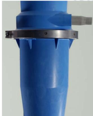
This Mid-cone Dilution Technology enables the CELLECO TWISTER hydrocyclone to have an elongated cone section for higher separation efficiencies without the need to operate the hydrocyclones at an elevated pressure drop.
