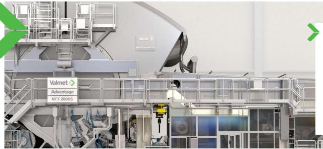
The NTT production line can be supplied in different machine widths from 2.8 m (NTT 100) up to 5.5 m (NTT 200).
