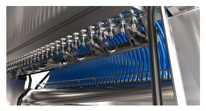
One of the most critical components on a tissue machine is the headbox. A properly functioning headbox enhances tissue makers' ability to produce various tissue grades at the desired level of quality.
