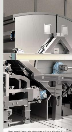
The hood and air system of the Yankee make up the latest Advantage Aircap design driving the hood temperature up to 550 °C and maximizing the drying area.
