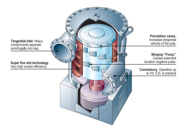
The HI-Q<sup>TM</sup> Fine Screen provides efficient and economical shive and dirt removal from a pulp stream under varied operating conditions in all kinds of screening systems. The HI-Q Fine Screen capitalizes on the advances in fine slot screenplate technology. The innovative Stingray<sup>TM</sup> Rotor makes it possible to operate at any accepts consistencies up to 4% on softwood and 5% on hardwood, while utilizing 0.2 mm (0.008") and 0.15 mm (0.006") or smaller slotted screenplates.
