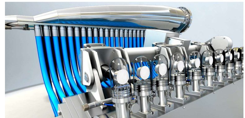
One of the most critical components on a tissue machine is the headbox
